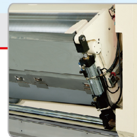
糊輪座可旋轉退出 Glue Unit By Rotation Way Eject
