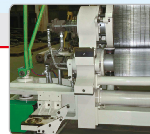
瓦楞輪採側吸設計 Corrugated Rolls Side Suction Design
